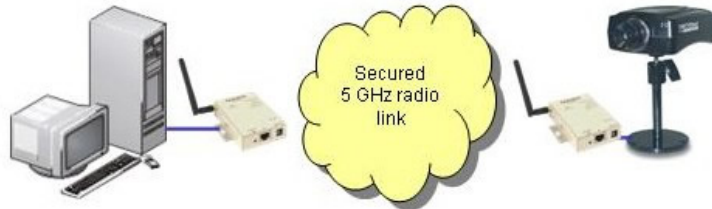
RJ45 ETHERNET CABLE REPLACEMENT BETWEEN TWO EQUIPMENTS
